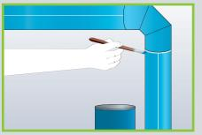
Seal all joints with Armaflex Adhesive. Do not stretch when sealing joints. When gluing joints under compression, with no gaps present, the wet adhesive method should be applied.
