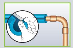
Locate the end of white release paper for the self-seal strip.
