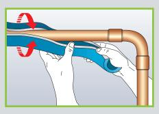
Open pre-slit Armaflex Ultima and snap onto pipe (the release paper is still protecting the self-adhesive strip).
