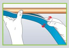
Adjust fitted Armaflex Ultima to ensure slit is easily accessible.
