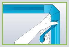
For additional security it is necessary to secure the longitudinal joints of Armaflex Ultima self-adhesive tubes with an additional Armaflex Ultima self-adhesive tape. Ensure that the surface is clean, dry and free from contamination, if necessary please clean it with Armaflex Cleaner.
