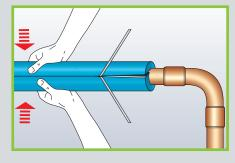
Close the slit seam and press together with firm pressure, to ensure a permanent seal.
